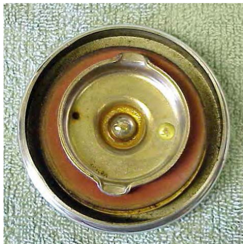
30-31 modified gas cap with a 6-32 screw epoxied into place opposite from the vent hole.
