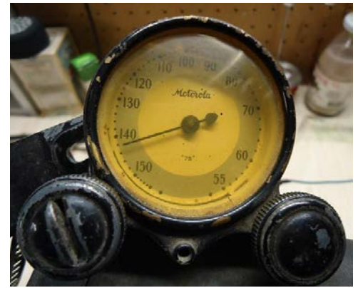
The world's first automotive head unit, the steering column-mounted tuner of a vintage Motorola radio. ( www.antiqueradiomuseum.org/thecarradio.htm )
