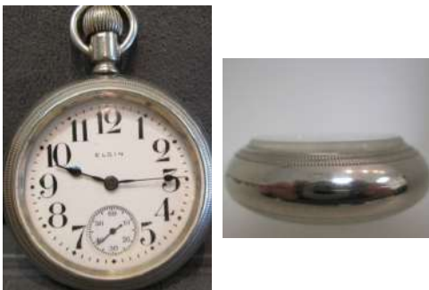
Pictured above is an example of what often occurred. The movement inside the case is dated 1929. The case, however, is from an earlier watch. Notice the taller stem, and the completely round bow. This case also is thicker. Pocket watches and their cases were interchangeable. If a watch
